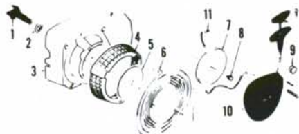
Fig. MC6-21 — Exploded view of left-hand rewind starter used on U.S. models and some export models.
