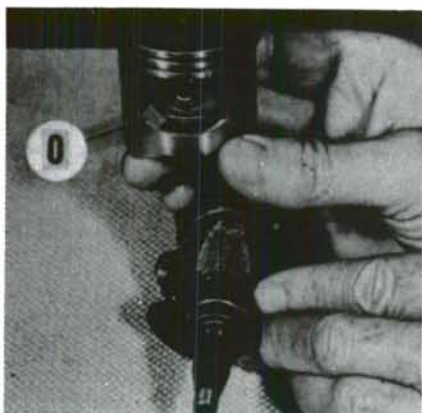
Fig. MC6-12 —Install piston so large offset (O) at piston pin boss is toward clutch.
