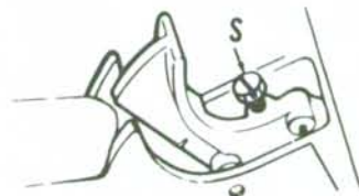
Fig. MC6-3—Fast idle adjustment on some models is performed by turning adjusting screw (S) on bottom of trigger.
