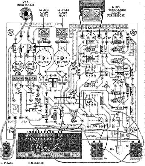
Fig.4: follow this wiring diagram to build the Digital Thermometer/Thermostat but note that only one buzzer is installed in the positions indicated (see text). Note also that PC stakes are installed at all external wiring positions and at the test points (TP). Q3 and its associated  $10 \mathrm{k}\Omega$  resistor can be omitted for panel meters with a decimal point driver pin (see Fig.8).
