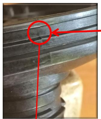
The problem seems to be on the tooling line, there is a small ridge Inside the o-ring seat, where the injection moulding tool is not quite aligned and leaves a small step. I think that could be the problem.
