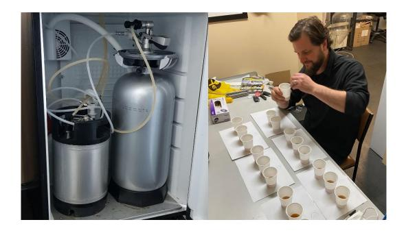
It is in the company's interest to prove that the two kegs provide the same beer-tasting experience. The statistical results in this report strongly support one-way PET kegs as a viable replacement for stainless steel kegs in the commercial beverage industry.
