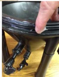
Add chilled wort and pitch yeast into bucket and then assemble cone onto the bucket.
