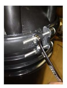
Tighten bolts to leave about 1/4 inch gap between rings.
