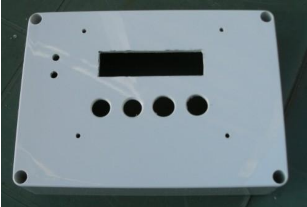
Cut out and drill the front of the box
