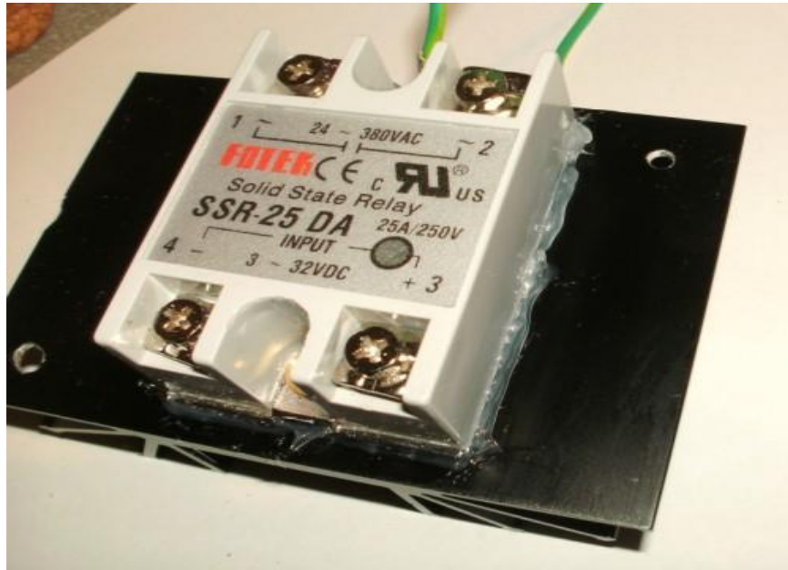
SSR and heatsink just before it is going to be mounted in the box
