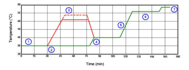
**Figure 1: 1**-mashing with water/grist ratio of 1:5 **2**-Mash separation (25-30% of thick mash and 70-75% of thin mash) **3**-Heating of the thick mash to 63°C and 30 min rest to activate  $\beta$ -amylase **4**-Mixing of both thin and thick mashes to achieve a temperature of 40°C and activate maltase **5**-Heating to 72°C to perform iodine reaction **6**-Heating to 78°C before transfer to lauter tun.
