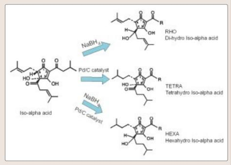
Figure 7. The production of reduced iso-alpha-acid compounds from iso alpha acid.
