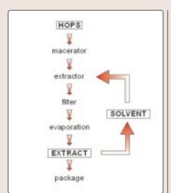
Figure 4. Process flow chart for the manufacture of hop extracts.
