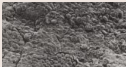
Figure 3. After – showing how the cell structure has been stripped away exposing the starch granules, which can now be degraded by enzymes during mashing.
