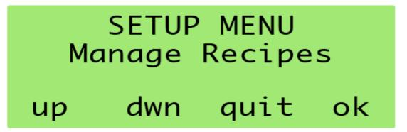
In this section is possible to save inside the controller memory up to 10 different settings for future use.
