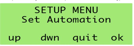
The basic principle of this configuration menu is the "step mashing" process. For each step user can configure target temperature (SetPoint) as well step duration. Moreover it's always possible to skip some of the steps according to the recipe schedule trough the START button.
