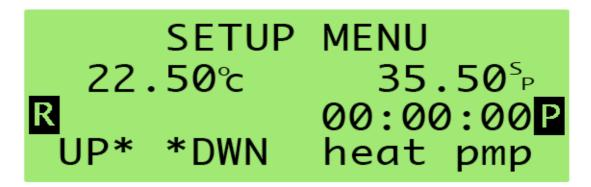
Manual process allow the user the full control of the entire mashing process by temperature settings and switch ON/OFF of both pump and heating element.
