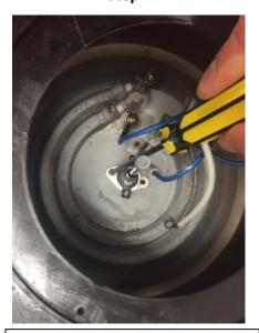
Unscrew the second screw that connects the thermostat to the boiler. Remove the thermostat from the boiler.
