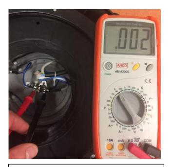
Connect the red and black prongs to the screws attaching the wires to the thermostat. The multimeter should 'beep' showing that current is running through the thermostat.
