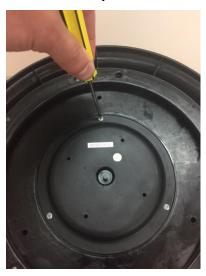
Use a screw driver to unscrew the bottom plastic cover, remove this cover
