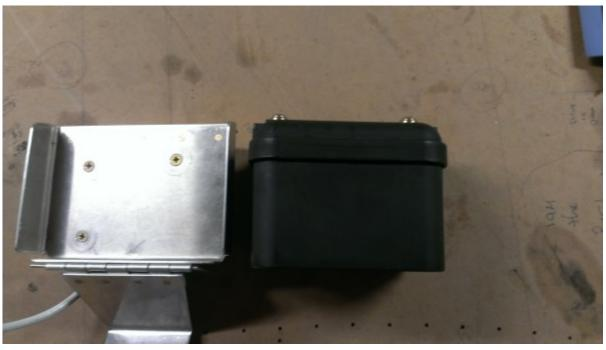
The pads are self-adhesive. I then covered them with a silicon tape which holds up to the operating temperatures.
