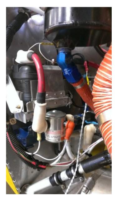
You can see the master and start solenoid which is going to replaced in phase two by the small ones on the bottom of the tray.
