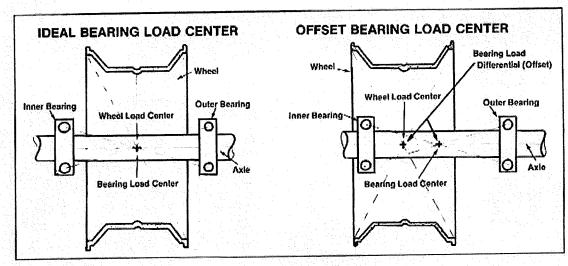
of a Honda Gold Wing, it works out this way: the axle and wheel bearing components are made of steel; the hub is cast from aluminum alloy. Obviously, steel is a much harder metal than alloy. Hammered with the same amount of force, the alloy will alter shape sooner than the steel.
