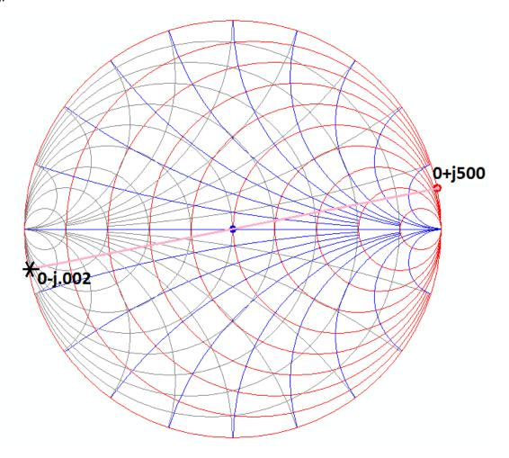
So, to go from 100+j200, we know we need an inductor in parallel to that load with a reactance of  $500\Omega$  and a series capacitor between that and the source with a capacitive (negative) reactance of  $150\Omega$ . At 1MHz, that comes out to about 1.061nF and 79.6 $\mu$ H. We just made an L matching network!
