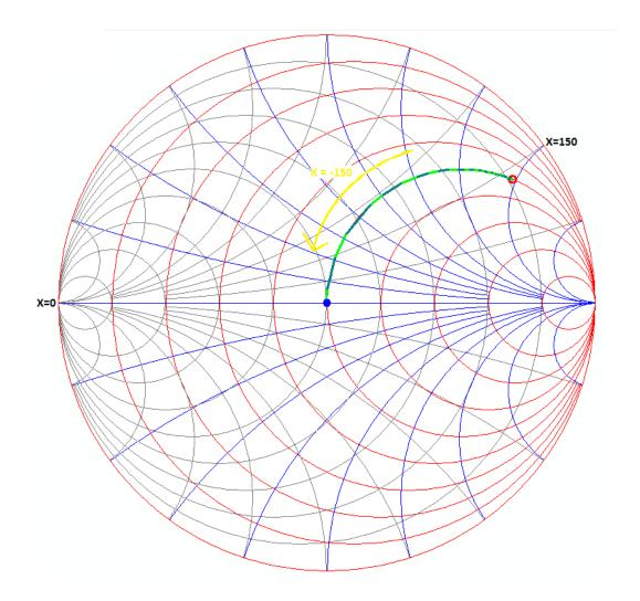
But what if we didn't start out on the  $50\Omega$  constant resistance circle. What if we started at 100+j200? What we would do then is simply follow the *constant conductance circles* with parallel components! Again, going up, so we need an inductor. This time in parallel. We need to go up **to** that red line we used last time because, again, it gets us to the middle with series components. From there, a series capacitor finished the path to the center like above.
