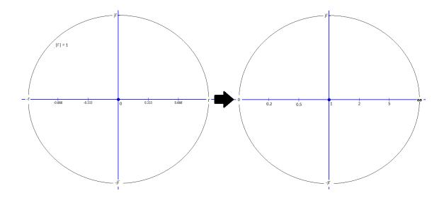
Now, lets say that those tick marks on the axis are tangent points of circles that have their centers coincident with the horizontal resistance line and midway between the tick mark and the infinity point. Grab a compass and draw them in. Then, lets get rid of that useless y-axis, we are done with it.
