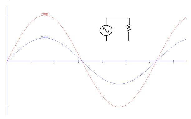
All that is fine and correct, but the problem is, a vast majority of us automatically make the assumption that when the voltage is at its highest, so is the current - and that is where the major problems start. They don't have to be highest at the same point in time!
