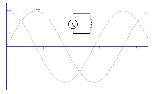
In other words, the voltage (E) on an inductor (L) leads the current (I) and, the current (I) in a capacitor (C) leads
