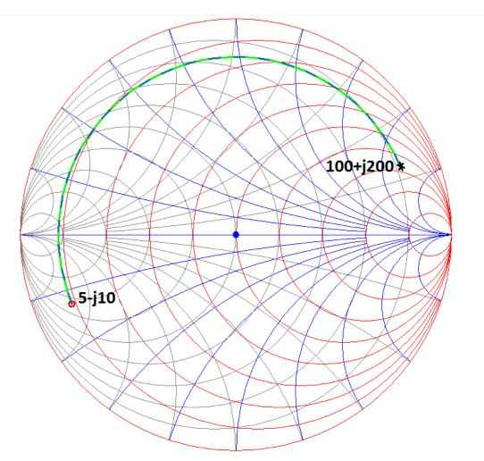
Thats how easy it is to calculate what a coax will do to an impedance value. Real coax has loss, and if you were to have a couple wavelengths of coax, you would see that circle spiraling inwards. On good smith charts, there is a dB loss scale that makes it easy to adjust for that on the chart. This is the first example of how a smith chart can solve a complicated math problem. The formula to do that, if you wish to try, is:
