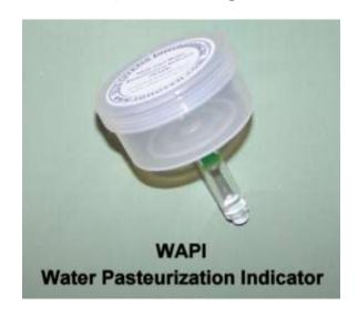
The WAPI was originally developed for use in third-world countries where clean water is scarce. It is very inexpensive and basically foolproof. While the device can't really be damaged by use, it would be a good idea to have a couple of them on hand, in case one becomes lost.
