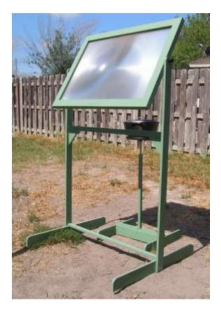
This type of solar cooker can provide an extremely high amount of heat, actually heating up the cooking area enough to cook eggs in less than a minute. I've actually seen pennies melted by the heat that this type of solar cooker can produce.
