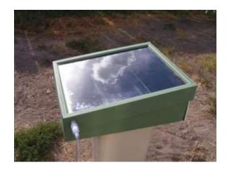
The inside of the box needs to be painted black for the best heat absorption. A clear glass baking pan (or two) is placed inside the box and filled with water. The device is left sitting in the sun to work. As the sun hits the box, it will heat up the inside, causing the water to vaporize. That water will condensate on the bottom of the glass and run downhill to the tube for collection.
