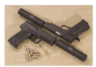
What most people refer to as "silencers" are actually suppressors. It is impossible to fully silence the sound made by a firearm, but it is possible to reduce it greatly. The degree to which it can be reduced depends upon more than anything on the speed that the bullet it traveling when it leaves the muzzle of the gun. Subsonic
