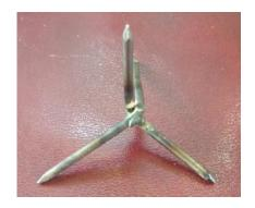
The caltrop in the picture is one that I made from a couple of 16d framing nails. I cut the heads off the nails and ground a point at that end. Then I bent them to a 105 degree angle. The final step was to weld the two nails together, to form the final caltrop.
