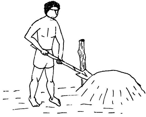
Fill to the top of this peg.
