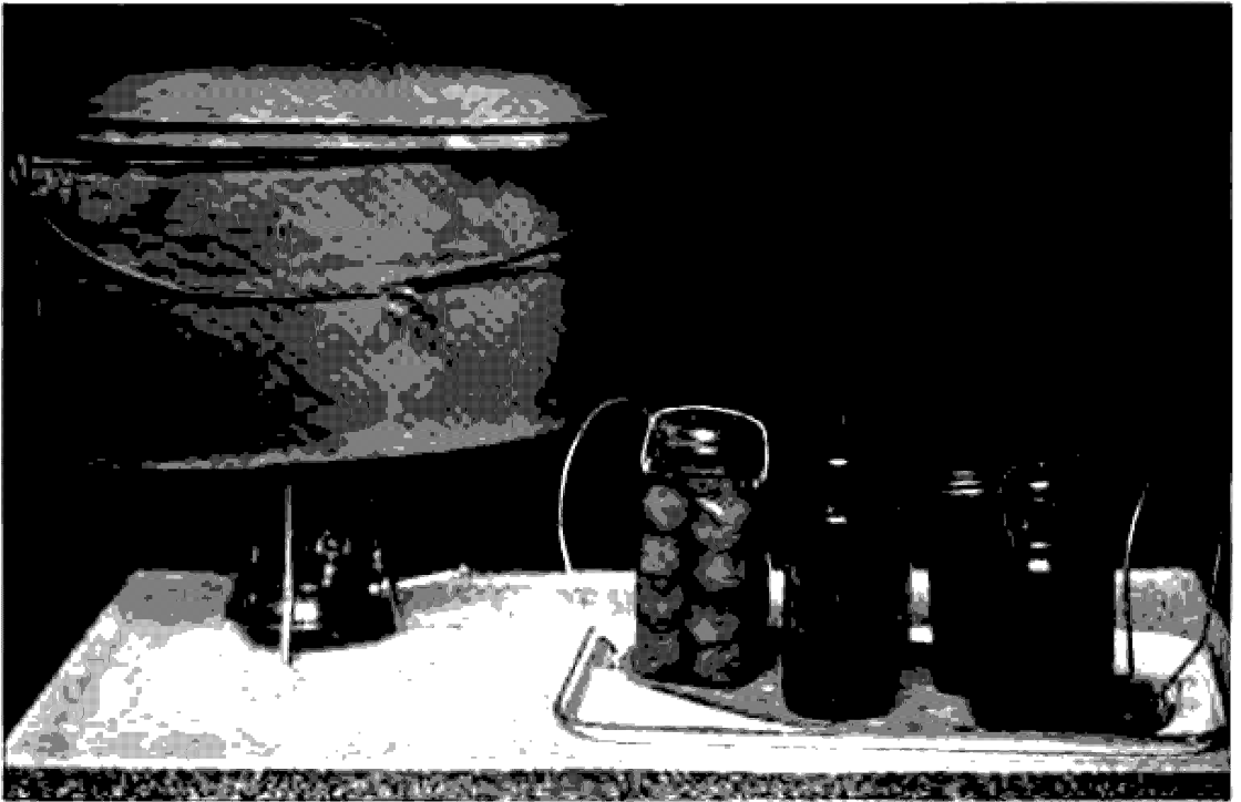
FIG. 19.—The processor and rack with jars ready to be sterilized. Note all clamps are raised and screw-top only partly screwed on.
