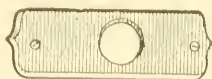
Fig. 190—Piece of Wood used to Secure the Knife in its Place and Admit the Tap.
