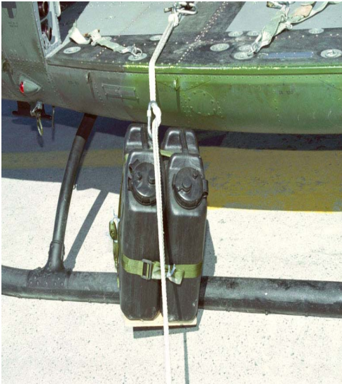
Figure 2-25: Bundle of Two Water Cans Ready for Rappel
