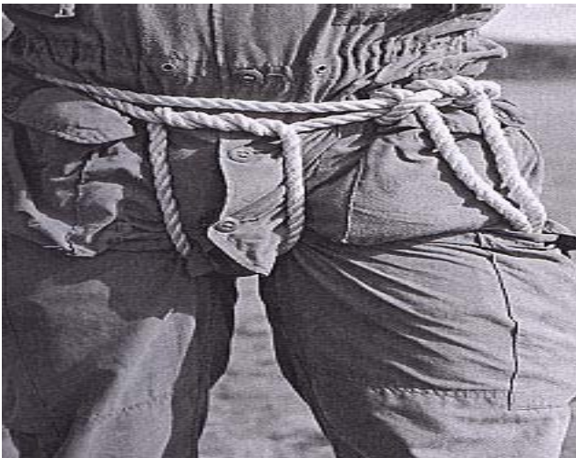
Figure 2-11: Swiss Seat Rope Stowage
