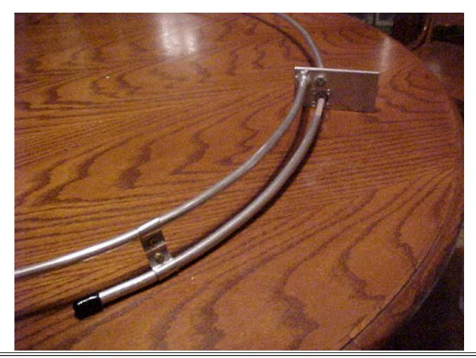
Position the 1" wide aluminum bracket on the Gamma arm, inward about 3 1/2". Expose about 3" of the RG-8 center section. This is just a starting point for matching this antenna. I was lucky and didn't need to make any further adjustment for lowering the SWR. The SWR on this design seen here, just the way it is, was 1.2 to 1 at 50.125Mhz.
