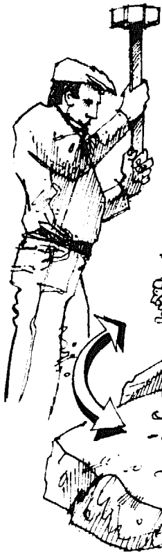
Making holes by hand with a plug drill
