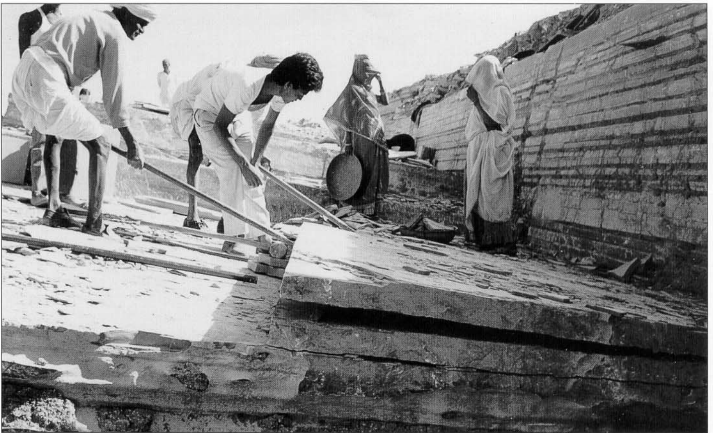
Figure 3: "Karstic features on joints and leverage with hammer leads"
