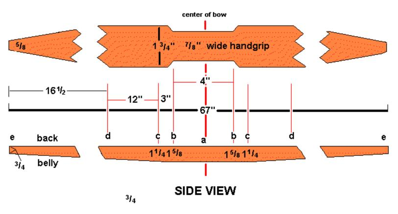
(NB, the bow is drawn to 67" length, designed for a 28" draw length. If your draw length is longer or shorter, alter the total length by 2" for every 1" draw length change (e.g. draw length of 26" gives a length of 63") Handle section (c-c) remains the same, the rest (c-e) should alter in proportion.)
