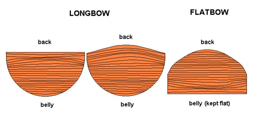
(the back remains flat, or slightly convex, following the natural line of the growth rings and the sides and belly slightly rounded into a "D" shape. Wood is shaved off with rasp, spokeshave, drawknife or scraper untill the appropriate tiller is maintained, all the time ensuring that the slope of the taper remains constant from handle to tip.)
