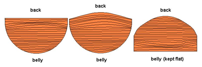
(the back remains flat, or slightly convex, following the natural line of the growth rings and the sides and belly slightly rounded into a "D" shape. Wood is shaved off with rasp, spokeshave, drawknife or scraper untill the appropriate tiller is maintained, all the time ensuring that the slope of the taper remains constant from handle to tip.)
