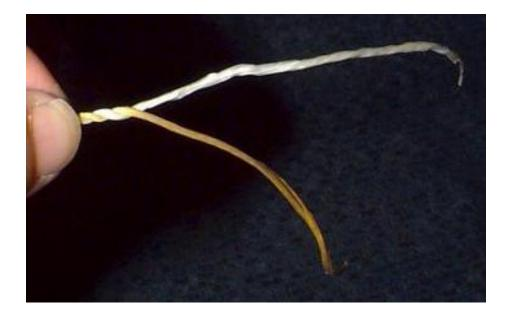
Form the loop as shown in Figure 6. Make sure you align the bundles as shown (same color over same color). Grasp the bundles at the bottom of the loop and twist the two bundles of same color together. Figure 6 shows white twisted onto white forming one large white bundle and yellow twisted onto yellow forming one large yellow bundle.
