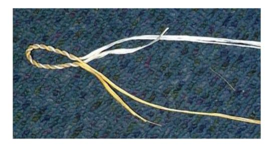
Holding these two bundles between the thumb and forefinger, perform the same twisting and rotating process until the last tag end of the strings have been braided into the bow- string. Your finished loop should look like that shown in Figure 7.
