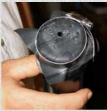
What I did was to cut up a section of Mountain bike inner tube into about  $4 \times 4$  inch sections with a  $5/16^{th}$  hole in the middle and lay that over the top of the tube reservoir and clamp it in place with a screw band clamp or a couple of winds with a rubber band.
