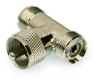
Here is pretty handy adapter a PL-259 to SO-239 T splitter. This adapter allows you to hook up two different antennas to your radio. For example I have a verticle intermediat range and a longer dipole. The vertical antenna transmission could be used for your local traffic and with the dipole aimed at your patrol location(s) like South of base camp.
