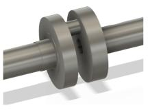
I used a dead centre held in another dead centre on the lathe although a 'wiggler' setup may have been more accurate. Total disclosure here, the first time I tried assembling the engine, the pin and the hole didn't mate and I had to bin and re-make the centre bearing. I wish I'd had someone to give me this tip before I started making mine <sup>(C)</sup>.
