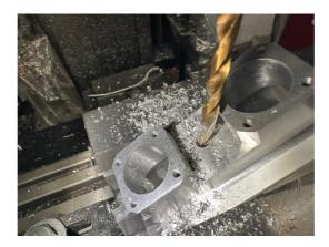
**TIP 4**: Use the hole in the centre bearing to mark out where the holes should be drilled in the centre crankshaft. I rotate the shaft to the correct angle (50deg BTDC) and use a sharp pin to bark out where the hole should be on the crankshaft. Make sure you file off any burrs after.
