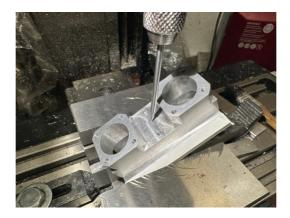
Start with an endmill to create a flat first, next use a centre drill to start the hole and lastly drill through with a nice sharp jobber drill.
