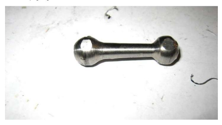
Now to try the HSS slotting mill cutter. And it worked better than any other metal, tried cuts of .2mm to .5mm and it cut very nicely. No sign of blunting the tool at all.
