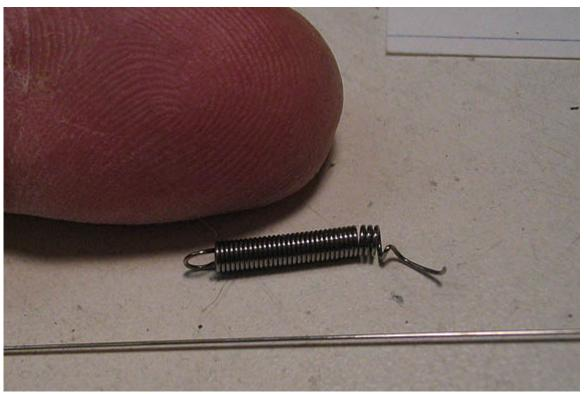
The two wire sizes I had on hand were both slightly different sizes than the original spring. One was almost .015", one about .0135". I'll make a few spring blanks in both sizes. I always make extras for a particular job, in case "someone" goofs.
