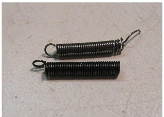
Here's the new spring, and the old one. In this shot, I'm just getting a sense of the position for the second eye needed on the other end. The eye pulling process is repeated. The new spring looks somewhat fatter in this picture. It's a trick of the camera, though. The new one is within .001" dia. of the old one.
