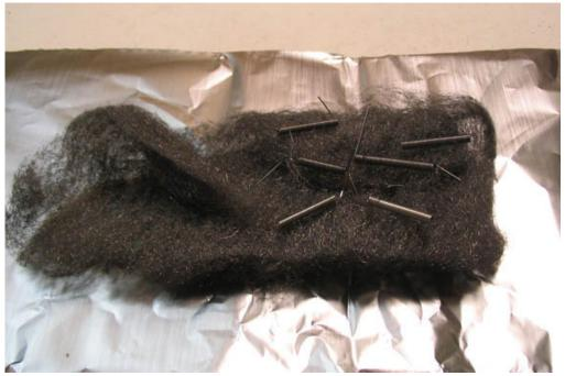
This next bit, including the following few pictures show the method I use to heat the springs. They have to be stress relieved after the winding process, or they won't hold their shape well. If you don't do this step, the springs won't be as springy as they should be, and can easily be stretched out of shape. I make a nest for them using steel wool and foil. Put the springs on one half of the steel wool.
