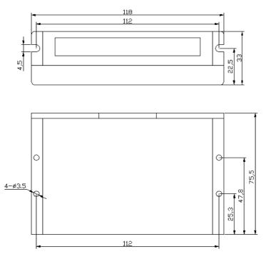
\*\*\*\* Recommend to use side mounting for better heat dissipation
