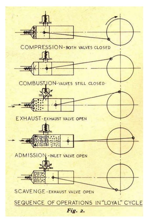
Mr Stone's diagram shows a fifth phase of operation, in which the return stroke of the piston produces sufficient increase of pressure to lift the exhaust valve a second time, and thereby scavenges or clears out more of the residual gases. My personal opinion is that this action is somewhat dubious, because the momentum of the incoming charge would keep it flowing till well past the outer dead centre, and if the pressure on the return stroke became high enough to lift the
