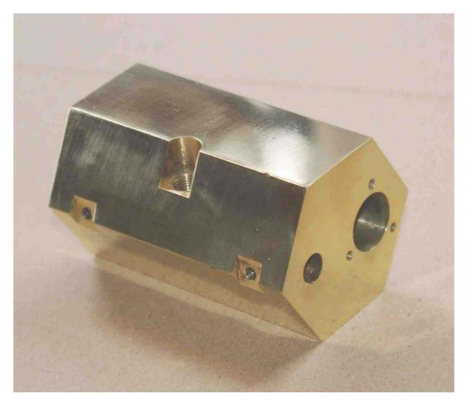
Sheet 15: CYLINDER BLOCKS - DETAILS OF AIR/STEAM INLETS
