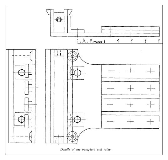
material is used, being shaped to slide' fairly tightly between the strips on the front plate. To this back plate another plate is riveted, being drilled and tapped to accommodate the 1/4 in. Whitworth feed screw which I turned from a short length of 1/2 in. diameter mild-steel bar, starting the thread by means of a tailstock die-holder, and afterwards finishing the thread with hand tackle in the vice.
