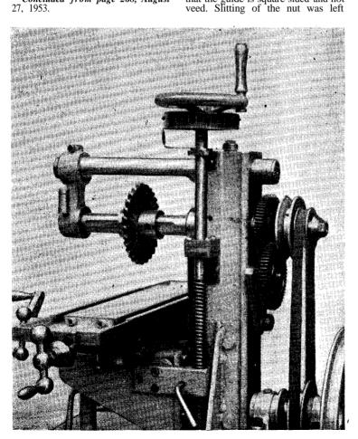
The machine set up for horizontal milling.
