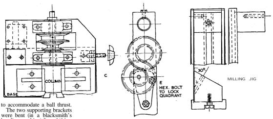
bending machine) from 1/4 in. thick flat plate and machined webs welded in place. A little tiling and scraping secured good seating on both faces, which is essential to avoid strain on base and column. Countersunk screws had to be used in two holes of the rightment hand bracket to allow clearance for elevating feedscrew block.
