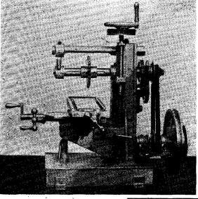
stud. When pivoted forward, the shaped point engaged a rack tooth. Saddle was locked and a cut made. And so on. Two strips were cut off plates and cleaned up. After screwing rack into place, the four holes to take table gib strip adjustment screws were drilled through rack and fixed strip in one operation. The rack is anchored to left-hand tray by a small bracket.
