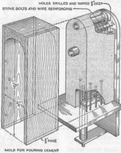
DETAIL OF MOLD AND METHOD OF REINFORCING
