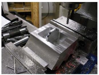
Machine the front and back of the block to size, 3/8 deep, leaving .005 inches for future machining. Drill and tap the holes to mount the oil pan.
