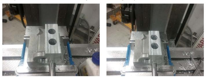
Cut the water jackets into the block. Drill holes to mount the head. Drill the hole for the camshaft setscrew.
