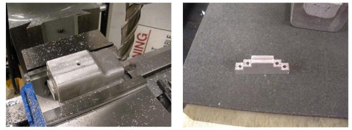
Next the block will need to be laid out. The absolute bare minimum (.060ish) was cut off to clean up the rear of the block. The block was then clamped down to the table flat on the bottom and the peak of the cylinder banks were skim cut just enough to leave machine marks.
