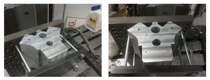
Insert a piece of 5/8 inch drill rod into the crankshaft hole. Laying the rod across the top of my vise gave horizontal alignment. Find the center of the cylinder bank and make a mark 5/16 inch on each side of center. Butt a square into the rod in the crank hole on both sides and align with 5/16 marks to assure vertical alignment. After aligning, use the pointer to pick up center of cylinder bank.
