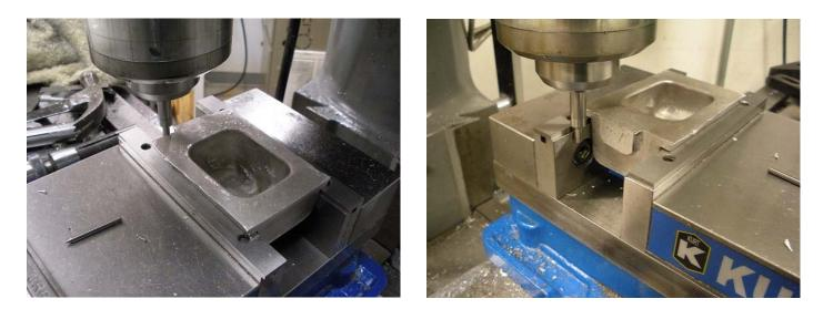
Tool Height was established by touching off the tool on the parallel and setting the DRO to -.200 inches. The parallels were then removed to clear the way for machining.
