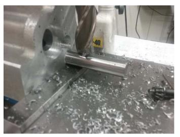
Machine top of cylinder bank to height leaving .005 inches for future machining. Use the edge finder to locate the front of the block.
