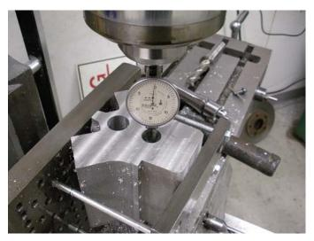
Drill the water passages into the cylinder banks. Drill the holes for mounting the bell housing adapter plate
