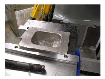
The edge finder was used to find the center of the casting both ways. Front and rear of the casting was used for center, left to right (X axis). The inside of the vise jaws were used to find center the other way (Y axis)
