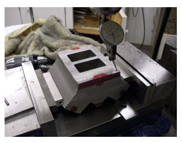
Pick up the center line with a pointed tool to find block center (Y0.000). Find center of the middle web of the block. Move .025 inches toward the front of the block. Use this point as the zero point (X0.000)
