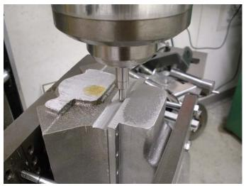
Use the edge finder on the oil pan flanges to find the center of the pan along the X axis. Double check by moving to zero X and Y axis and make sure the edge finder appears to be center of the pan and centered on the split.
