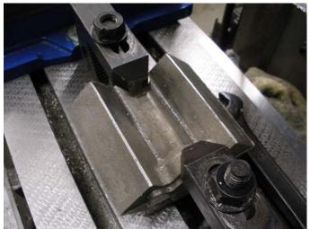
The block was then rotated bottom up and a bare minimum skim cut taken to clean up the bottom. The distributor boss was just cleaned up with a few strokes of a file.
