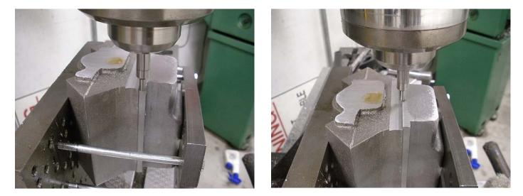
Machine the front down .005 past the machined surface at the bottom of the block. Drill the crankshaft hole to  $\frac{1}{2}$  inch and drill the camshaft hole to  $\frac{5}{8}$  inch
