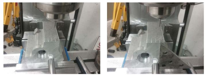
Indicate the bar at the front and back of the block to assure alignment along it's axis. Touch your cutter off the top of the rod. Set Z axis to .3125 inches.
