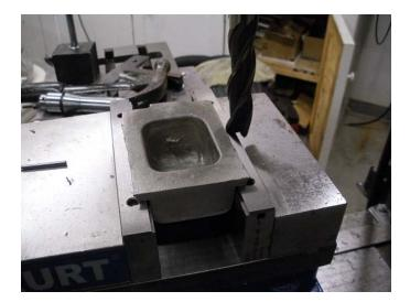
The top surface was machined down until the DRO read zero. Now the side flanges should be .200 inches thick as per the drawing. The side of the flanges were milled so the pan is 2.600 inches wide.
