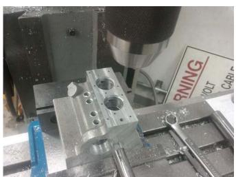
Rotate the block to the other bank and repeat the process.
