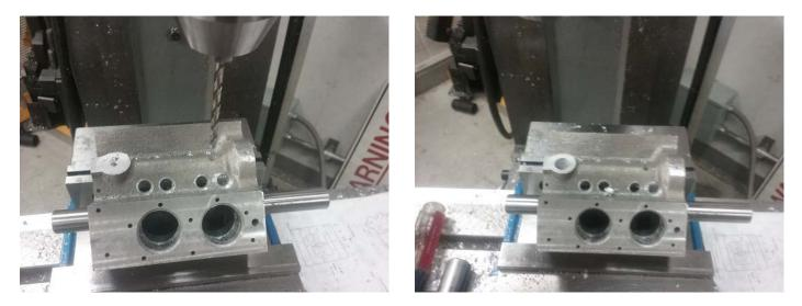
Finally drill the hole that locks down the distributor. That's all for the block and oil pan. If you haven't already, tap all the holes that require threads.
