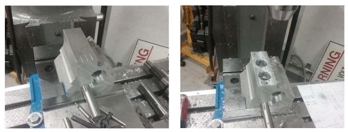
Machine the distributor boss to the correct height. Insert a <sup>3</sup>/<sub>4</sub> inch piece of stock or tool bit into the camshaft hole and use it to locate center of the hole. This is also center of the distributor hole.
