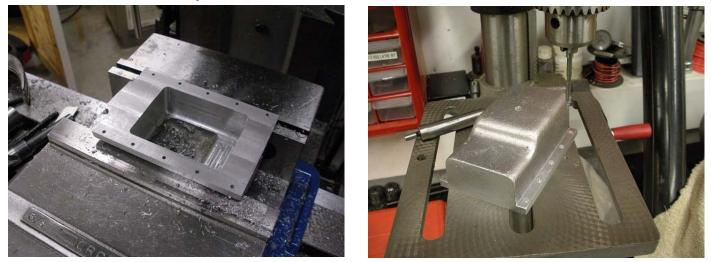
Finally the pan is rotated bottom up and surfaced so that the drain plug washer will seal. Take the absolute bare minimum needed to clean up around the drain hole. Next you will need to machine the center bearing support. Machine the part using .250 inch thick stock. Do not reduce the thickness of the support at this time.
