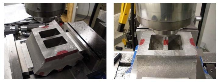
Machine the bottom surface down to the horizontal line. Drill and tap the holes to mount the main bushing support.
