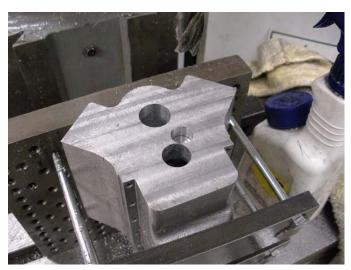
Use the boring bar to finish off the gear pockets. Drill all the holes for the mounting of the timing cover, water pump, and idler gear. Be careful that the three holes up each side of the timing cover are not in a straight line.
