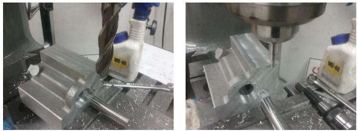
Drill the cylinder holes to <sup>3</sup>/<sub>4</sub> inches. Finish boring and counter boring the cylinder holes.
