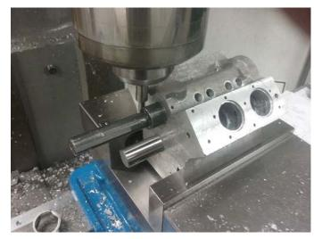
Spot drill the distributor and crankcase vent. Drill the hole for the crank case vent. Drill the hole for the distributor. Be sure to be centered on the camshaft for proper gear mesh.
