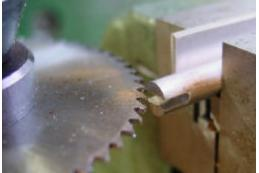
Cut the slot in the piston rod.
