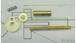
The crank is made of the 2 layers of tube, a cut off 6-32 screw. The screw needs to have some of its threads filed down to fit in the first tube. Now is the time to drill the axial hole in the screw
