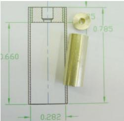
The cylinder is a tube with an end cap made to accept the copper tubes.
