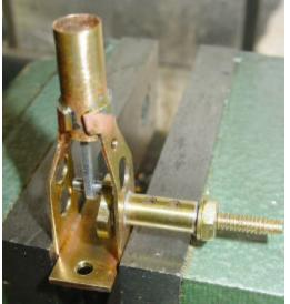
Solder the cylinder in place so there is .015 gap inside the cylinder at TDC.
