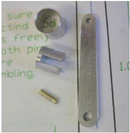
All the piston parts. When the tube is glued to piston center the wrist pin is captive. The connecting rod is tapered to allow it to move over a wide enough angle for the crank.
