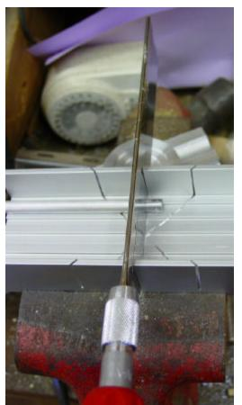
Use a razor saw and miter box to cut the tubes. Be sure to debur everything.
