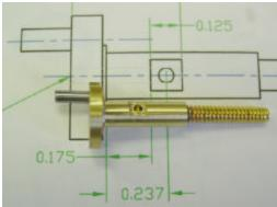
Make the small exhaust flat. Drill the hole to the center hole.
