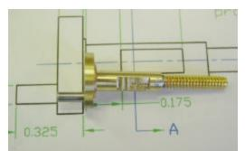
Flip the shaft and make the longer input flat.
