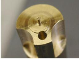
A length of brass had the hole for the crank pin drilled and 2 cuts made for some balance.
