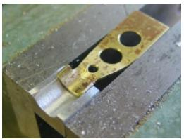
The frame sides are cut out. A concave form is made to make the curved areas.
