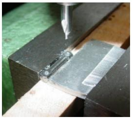
Center drill, drill and ream connecting rod holes.
