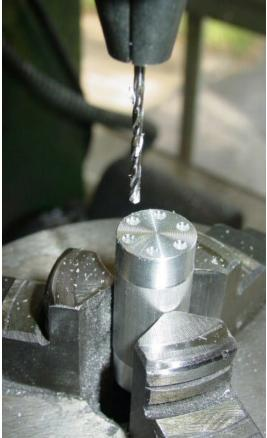
Drill bolt holes in head.
