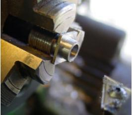
Keep inside flange long to hold in chuck while drilling head and exhaust holes. Turn to length later. The ID needs a champher for connecting rod clearance.
