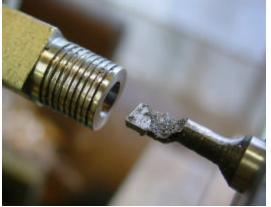
Fins were cut with a slitting saw blade held like a cutter. The bore was drilled slightly undersize. Counter bore was added for the valve disk. The Inside was honed with 400 grit lapping compound until a section of ¼ drill rid fit in, then that was lapped to perfect fit.
