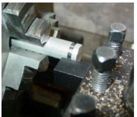
Tube bender, turn a grove the size of the copper tube to bend and move the end of a tool up to the grove.
