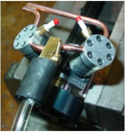
The throttle was a last minute idea. It joins the supply tubes, looks like a carburetor and throttles the speed some. The rubber tube coupling works but not well enough. At 40 PSI it pops off a lot. The trumpet should have had a sharp edge to hold the tube.
