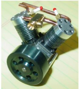
Finally it is complete. With the throttle, plugs and exhaust pipes. It runs great and has a different sound with the V timing.
