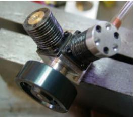
Test each cylinder separately to see it runs. About 50 PSI was needed at first but after 30 minutes it ran great on 35. Don't forget lots of oil at first.
