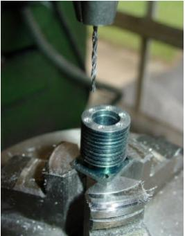
Drill bolt holes in cylinder. If it is done in the same setup the holes will be
