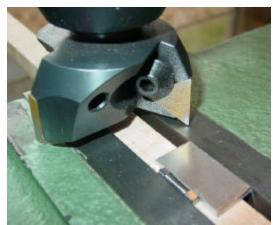
Mill flat sides on connecting rod.
