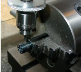
Center drill exhaust ports to keep fins and curved surface from causing the drill to wander...
