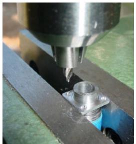
Drill the mounting holes. Later using a 1/16 diameter burr, angle and elongate the holes so the screws will enter.
