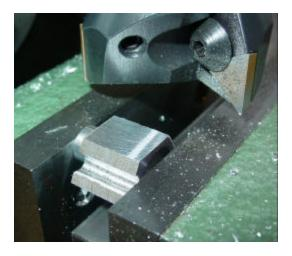
Drill 2 holes to start side flutes and mill to size.
