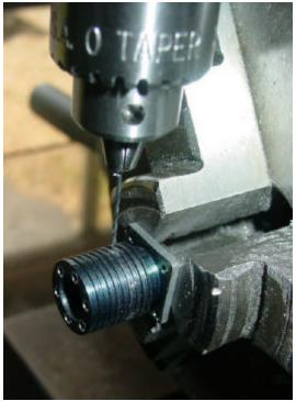
Drill exhaust ports. Be sure to align them with the flats on the cylinder so ports line up
