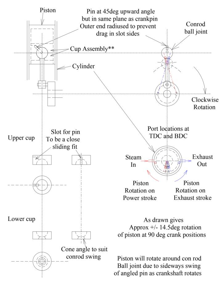
\*\*Cup assembly soldered inside piston after assembly with conrod
