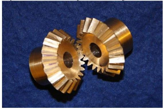
The photo below shows the teeth meshing at the large end of the gear.
