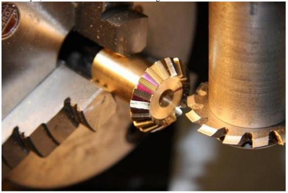
After the first cut, we have a parallel gap with tapered teeth. These will not engage with each other because of the difference. What I need to achieve is a tapered gap and tapered tooth that will mesh along the complete tooth profile.
