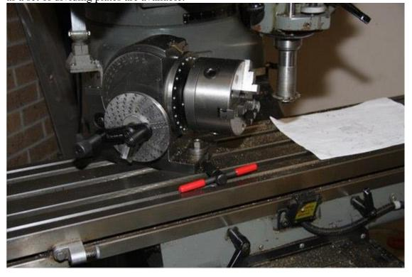
The next step is to choose the cutter to be used, I use normal spur gear cutters. If I was cutting a spur gear with 20 teeth, the cutter chosen would be a No.3, but in the case of mitre gears, a cutter to suit a larger number of teeth is chosen. This is because we use the PCD at the larger
