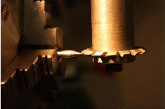
The index pin is set in a dividing plate with an even number of holes, this suits my dividing head which has a ratio of 40:1. This means that with 20 teeth, each tooth will be 2 full turns of the handle. The first cut is made to full depth.
