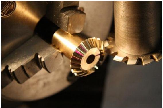
The photo below shows the teeth meshing at the small end of the gear.
