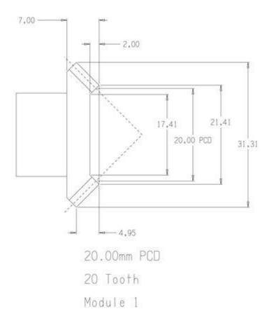
The mitre gears to be cut are Module 1, 20 tooth, 20mm Pitch Circle Diameter. The first thing to do was draw up the gears to find out the sizes required. Rather than go into a detailed explanation as to how the sizes are achieved, I have included a drawing of the finished part.
