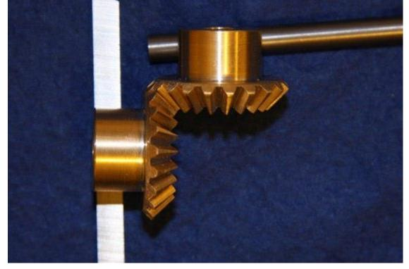
The above procedure is applied also to cutting bevel gears, allowing for the different angles involved.
