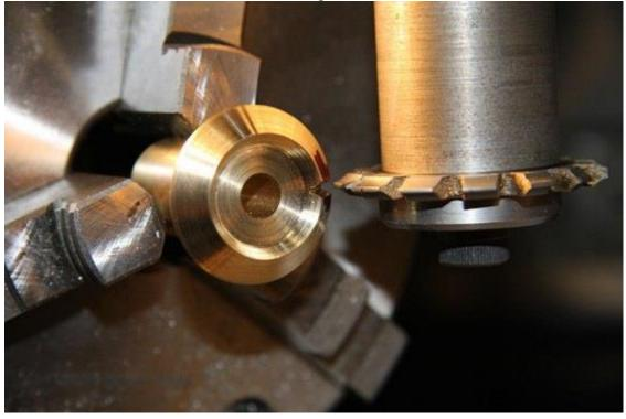
The next tooth is indexed by turning the handle 2 full turns and re-engaging the index pin in
