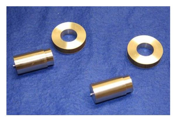
The shanks were stood on end and the larger piece sat on the end held by the turned step. These were gently heated from underneath the large diameter and resin cored solder applied from the top. When the solder flows down towards the shank, remove the heat. The parts were allowed to cool and then machined to size.
