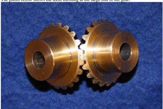
And here we have a photo of the gears intersecting at 90 degrees. The shanks have been trimmed down to the length required and burrs removed from the teeth using an abrasive
