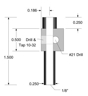
The carburetor body is made 1.5" x 0.5" x 0.375" brass or aluminum. Length may vary depending on application.
