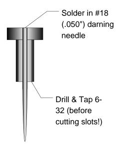
The needle valve is made from 3/8" brass rod and a #18 darning needle. Use a piece long enough to chuck it in the lathe and do the machining, drilling and tapping before separating the part from the stock rod.
