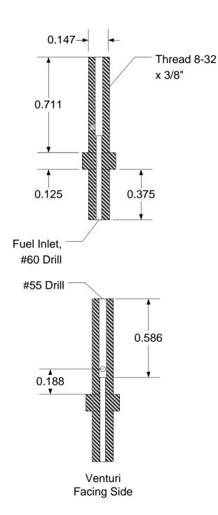
Jet is made from 3/16" or 1/4" brass rod approx 1.125" long. The through hole is best drilled on a lathe.
