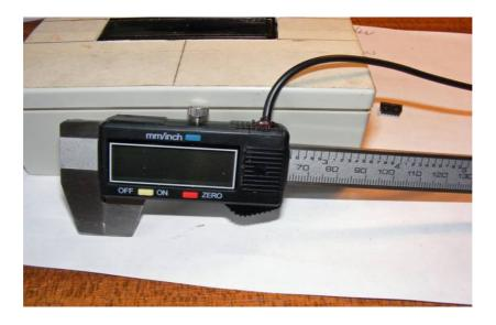
This is the finished calliper. The calliper is now powered from the remote screen box with no need for a battery. Most of these callipers carry on running after you have switched the on/off button to off. All this button does is turn the screen off, so it is a good idea to remove battery on your callipers when they are not going to be used.
