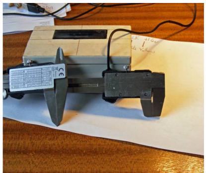
Original calliper on left,,, modified on right to fit onto my lathe, also you can see the screws that are hidden behind the metallised label...
