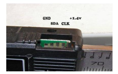
This picture shows the data socket with little cover removed and connections as they are on my calliper.
