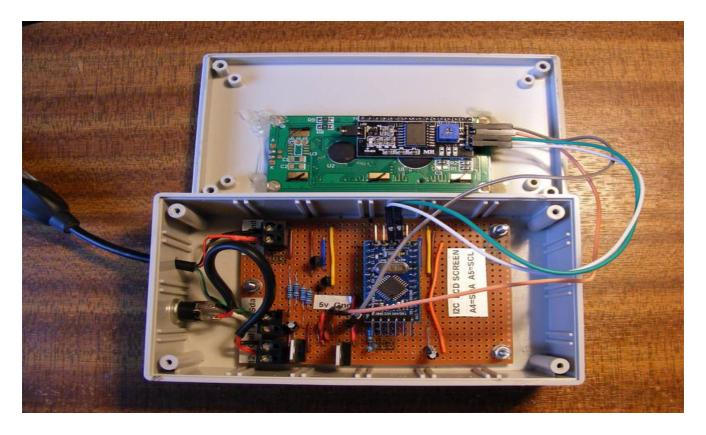
Modified Calliper and display being tested before fitting.
