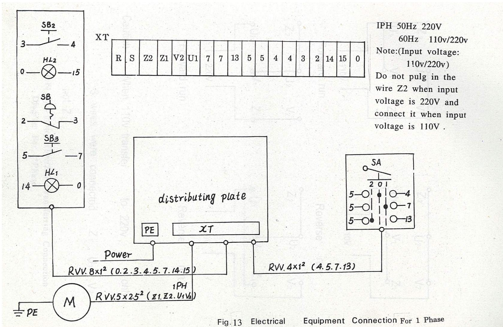
Fig. 13 Electrical Equipment Connection For 1 Phase
