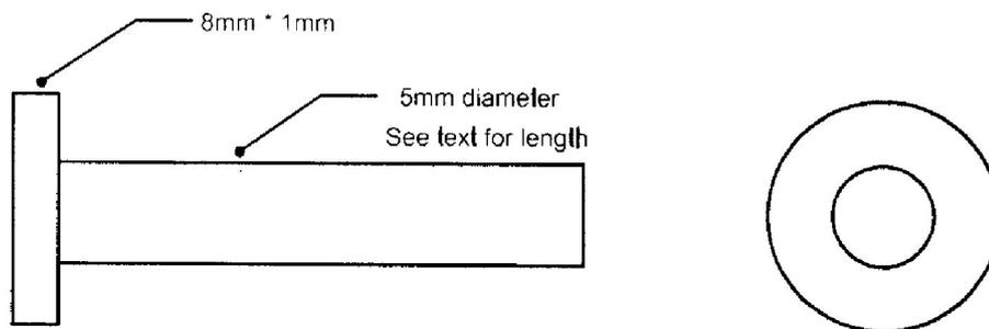
Note that there is no measurement on the length of the new core. This ideally should be about 3-5mm past the end of the coil former but it depends on how you make your coil enclosure. My friend George Punter will be making his by using a 3D printer. In this instance the plan is to have the coil assy. slip into the new casing which will incorporate the mounting lugs. Note:- not a good idea to use a steel bracket, rather use plastic or aluminium etc.
