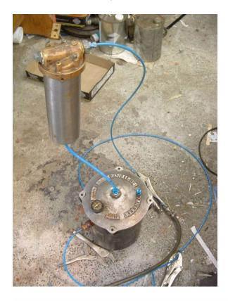
Rig with pressure to upper vessel, intermediate pipe open and vacuum to lower vessel (pipe previously connected to upper vessel was pinched off and removed before opening the vessel)
