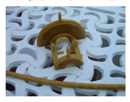
Here's the part removed from the mould "warts and all" there are two very tiny bubbles in the tips of the two tallest risers but note the bubbles in the leader scrap I came perilously close to blowing air into the mould probably because I got all out of sync taking photos screwed up my usual routine I let the air in way too fast and it "ratholed" sometimes you get lucky, sometimes you don't.
