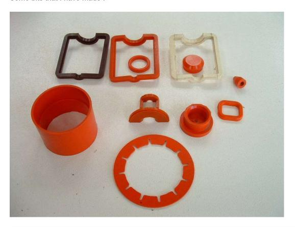
Polyurethane can be gravity cast into open moulds (degas mixture in a vacuum pot before pouring) or injection moulded into a closed cavity mould.
