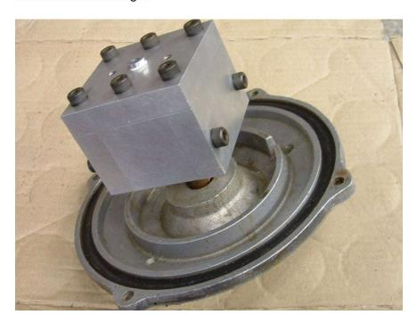
The mould, upper vessel and connecting pipe are coated with release agent I use a brush for the mould surfaces and slosh some around in the upper vessel and drain it out via the pipe.
