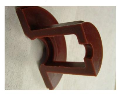
This is the finished part, riser sprues & flashing removed. It's a custom seal for Nitrogen pressurizing shockabsorbers (I designed the filling machine).
