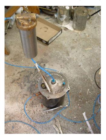
The pipe between the vessels is then pinched closed with vice grips and the vacuum closed off at the lower vessel (no point in losing the vacuum you have already built up).
