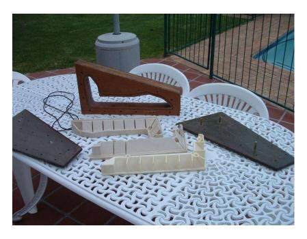
An MDF cavity with draw angle (liberally laquered to seal), steel plates, "O" rings etc. Silcone was first cast around sample part in the cavity. Silicone cut to split line with a scalpel (plan ahead) and subsequent parts cast in rigid clear (pigmented to white translucent) polyurethane.
