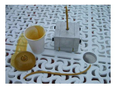
Here's the mould removed you can see the weeping it does not seal entirely (this is not injection mould standards here flycut aluminium).
