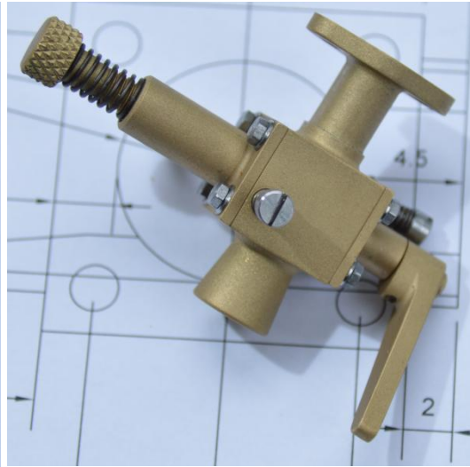
Wyvern carb based on Stride/Rupnow design – light sand blast finish
