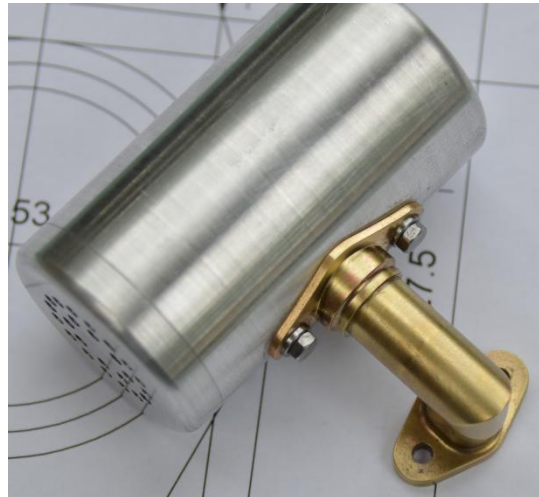
Silencer showing use of solder rings. Coupler made from 4 parts – light polish
