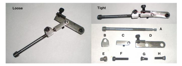
(In the above pictures of the assembled linkage the screw (H) is shown back to front.)
