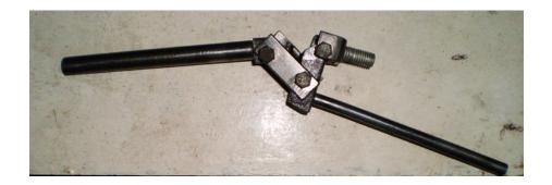
The basic imperatives of my design was that the lathe itself was not to be modified in any way, but that the new tensioner should use the same anchoring points as the original tensioning stay.
