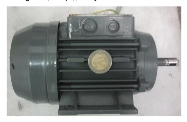
The Ø26mm coin is for size comparison. This is a very small motor for 1.2kW. The rewind cost a couple of percent the price of an off the shelf high speed motor. An acquaintance who imports high speed fan drives decided to see if he could reverse engineer a motor based on the above.
